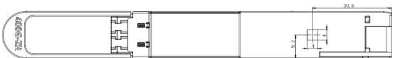
Figure 9: Case Temperature Measurement Point (All dimensions in mm)
