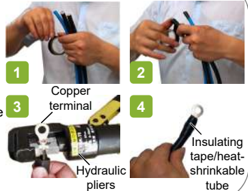
PDP protection earth ground cable
