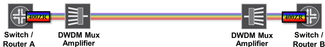
Figure 4 Router switch line card with 400ZR DWDM Interfaces
