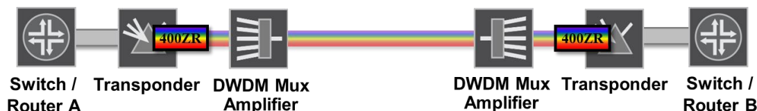
Figure 5 Transponder Line Card with 400ZR DWDM interfaces
