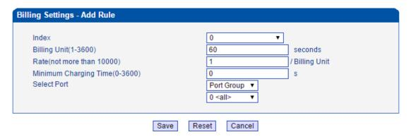
**Minimum Charging Time**: set minimum charging time, some operator does not charge if the call is less than some seconds when call is connected, user can set that value here. If the operator starts billing once the call is connected, please set 0 here.
