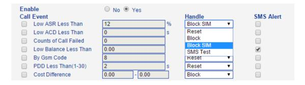
**Low ASR Less Than**: This value is the threshold of the ASR, once the exact ASR is lower than this value, the UC2000 port will be considered as the low ASR.
