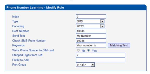
For make sure the configuration work, we can use the Matching Test. Input the "Your number is 8618344144906" at Test SMS Text, press the Test, you will get the match result.
