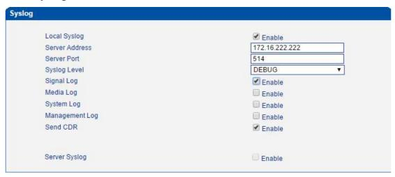
Syslog is a standard for network device data logging. It allows separation of the software that generates messages from the system that stores them and the software that reports and analyzes them. It also provides devices which would otherwise be unable to communicate a means to notify administrators of problems or performance. There are 5 levels of syslog, Including NONE, DEBUG, NOTICE, WARNING and ERROR.
