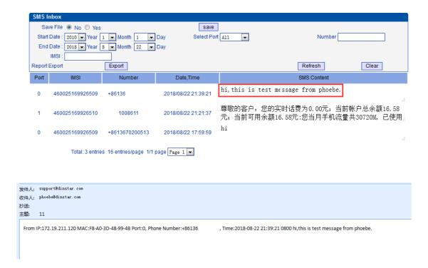
The UC2000 series gateway support to send the SMS received on the gateway to user's mail box. Login device's web, go to **SMS and USSD-->Email** page, enable SMS to Email function, and configure the other parameters needed.
