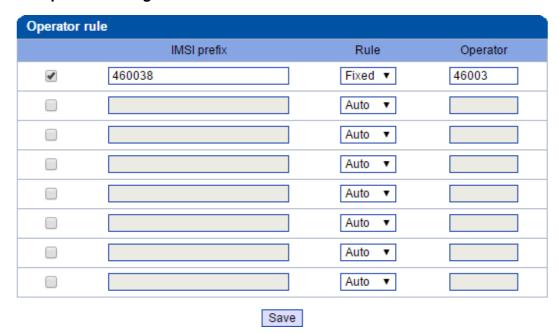
Operator configuration aim to set operator code for batch of SIMs. Inserted SIM cards will match with IMSI prefix and register SIM card to the code as per setting.
