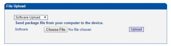
On the **Tools**  $\rightarrow$  **Firmware Upload**, you can upload a firmware to upgrade the device. But you need to restart the device for the change to take effect.
